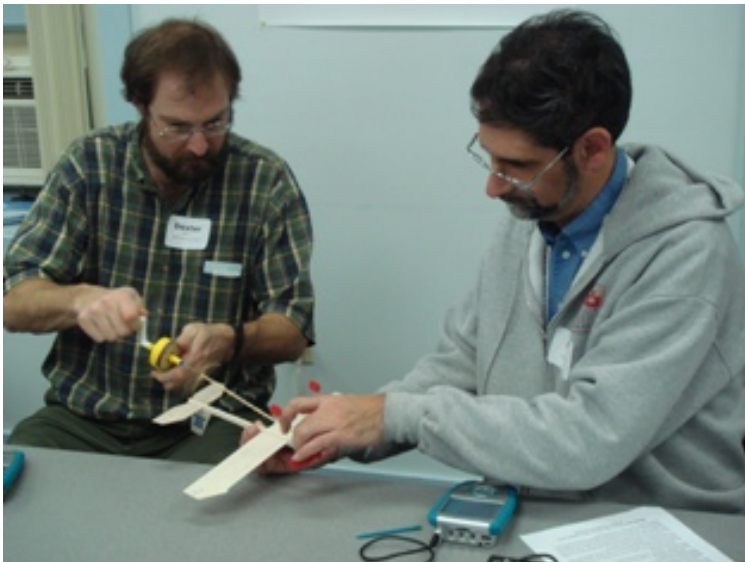
Measuring force exerted by rubberbands in model airplanes.
